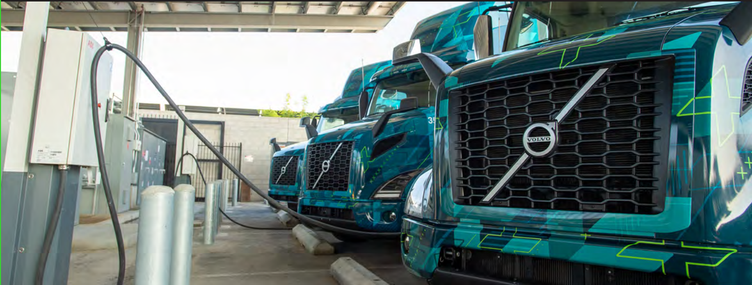
Caption: Three Volvo VNR Electric trucks charging at Dependable Highway Express' facility in Ontario, California.
